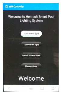
On the controlling page, you can press "Turn off the light" to turn off the lights, and press "Turn on the light" to turn on the lights. Press "Switch to next show" to switch to next program of the lights. Press "Choose Color" to select a program you want, and wait for some seconds before the lights switch to that program.
